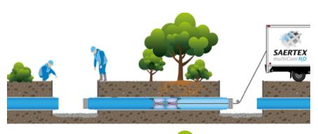
4. The rehabilitated pipe is reconnected and service is restored
