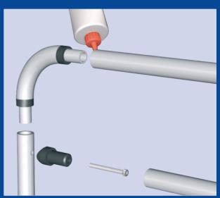
Standex Cobra PC has the same dimensions as 1", 11/4", 11/2" and 13/4" tubes. The dimensions can be connected using the AC plugs. Connections are fastened with 2-component glue, while plugs for vertical tubes are fastened with special bolts.
