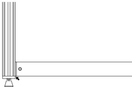
5. The lower edge of the cross rail is adjusted to the upper edge of the plug of the upright.
