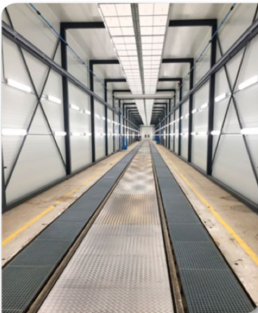
Example: 120 m long spray booth with more intermediate roller doors. Doors are not visible when open.
