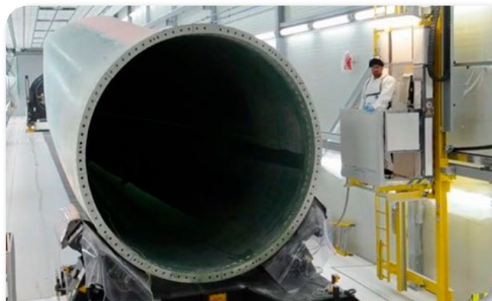
100 m long spray/drying booth with zone-ventilation according to EN 16985. Energy consumption is reduced to 1/6 without compromising on safety.
