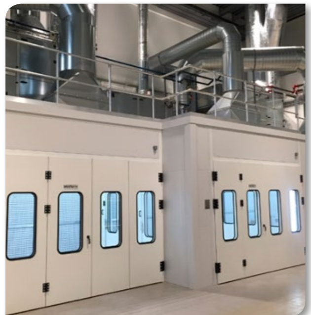
Above: Kongsberg Defence & Aerospace, Norway. 3 spray booths with horizontal ventilation.
