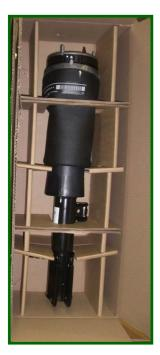
These units are combined shock absorber and air spring assemblies and are proving to be a commonly replaceable part on these vehicles; we are already seeing a large demand for the genuine units!
