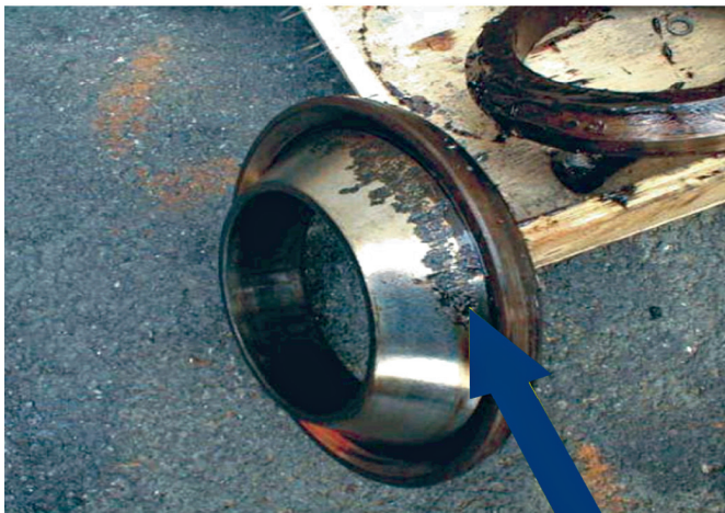
Distress increased from 4 to 26 however FFG Vibration MISSED this!
