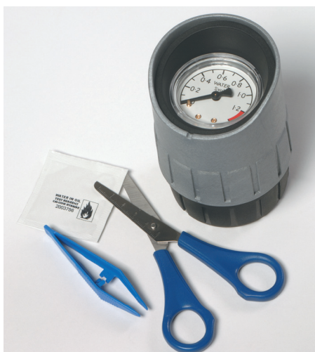
ECON Water Test Cell
